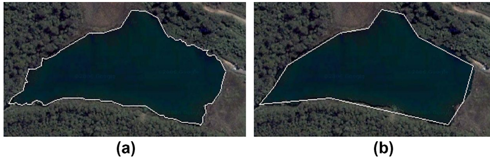
Fig. 3. (a) Polygon representing a lake. (b) Simplified polygon representation.
